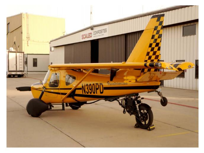
The ground mode is shown above. When it's time to fly the wings fold forward and the rear drive assembly is disconnected and stored in the rear seat compartment.
