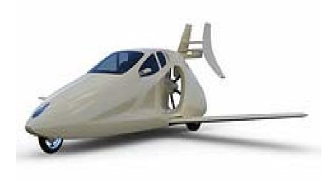
The wings fold under the body and the rear tail becomes "tight" to the body for ground operation.
