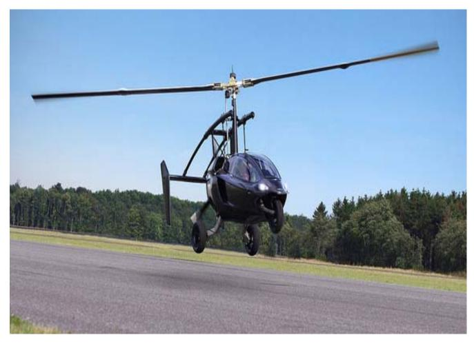
For ground operations both the rotor and rear-facing prop fold as the tail and the support members become "tight" to the body.
